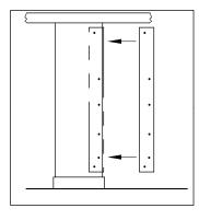
4. Drill 3/16" diameter x 7/16" holes (Do not drill thru). Attach 1001375 Strip Bracket onto 3/4" U-Channel using 1002499 Torx Screw. Place Strip **Bracket on inside** of toilet stall.
