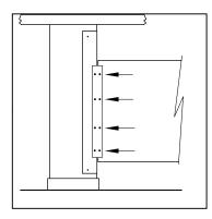
3. Use 1002665 **Button Head** Screws - 5/8" and 1002666 Sex Bolts in topmost and bottom-most holes to secure **U-Channel Bracket** to stile.
