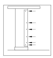
5. Drill 1/4" diameter holes through 1/2" thick panel using hole pattern of Strip Bracket (mounted to U-channel on stile) as template.
