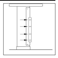
2. Drill 1/4" diameter holes through Phenolic (top and bottom only). Use holes on U-Channel as a template.
