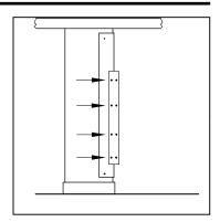
Drill 1/4" diameter holes through Solid Color Reinforced Composite (SCRC) material. Use holes on U-Channel as a template.
