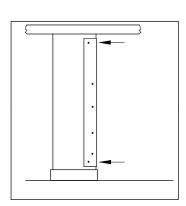
5. Drill 3/16" diameter x 7/16" holes (Do not drill thru) on 1/2" thick panel using hole pattern of Strip Bracket (mounted to U-channel on stile) as template.
