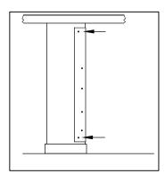
6. Use 1002499 Torx Screws - 7/16" to secure Strip Bracket to 1/2" Thick Panel.
